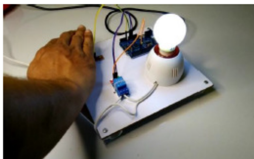
Figure 4.2 LED is ON when the object is detected
